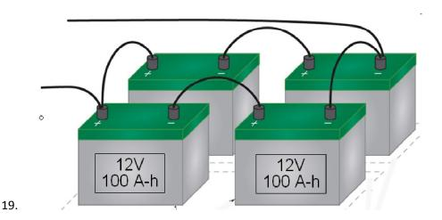
What is the output voltage and output current of the battery configuration above? Assume all batteries have the same voltage and capacity.
