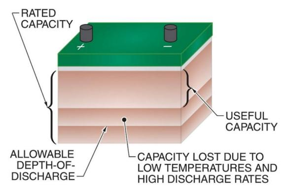
Due to the allowable depth-ofdischarge, low temperatures, and high discharge rates, the amount of useful output in a battery bank is less than the rated capacity.
