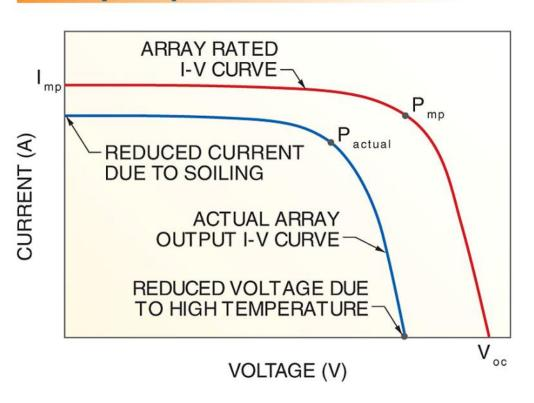
Actual array output is often less than rated output due to soiling and high temperatures.
