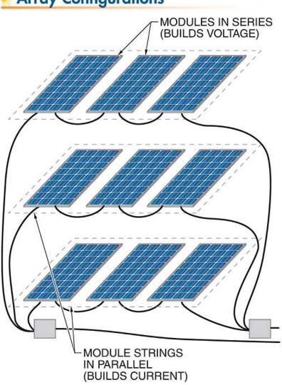
Modules are configured in series and parallel to match the array rated capacity needed to produce the required output.
